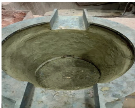
Figure 3. Appearance of the casting ladle with a chamotte-based protective refractory coating prior to pilot-industrial operation.
