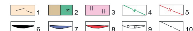
1 – lava breccias of porphyry of the Talovskaya suite; 2 – siltstones -a and diabases b of the Gerikhovskaya suite; 3 – porphyry; 4 – porphyrites; 5 – plagiogranite-porphyry; 6 – copper-pyrite ores; 7 – copper-zinc ores; 8 – polymetallic ores; 9 – disseminated polymetallic mineralization; 10 – veinlet-disseminated copper mineralization
