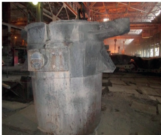
Figure 1. General view of the casting ladle used in Smelting Shop No. 1.
