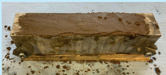
Figure 2. Casting of backfill UCS samples.
