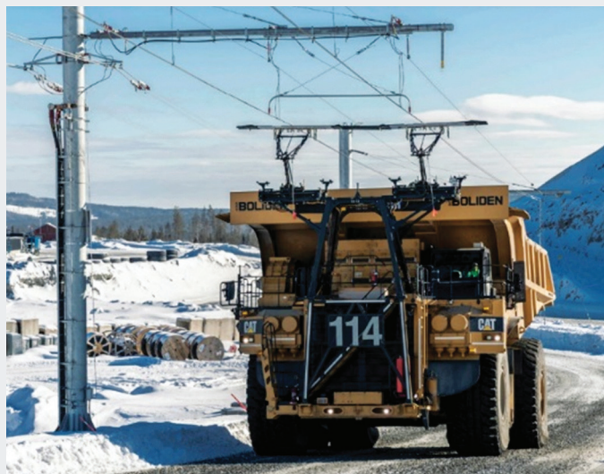
Figure 1. Trolley Assist truck run in Aitik iron ore mine of Boliden in Sweden.
