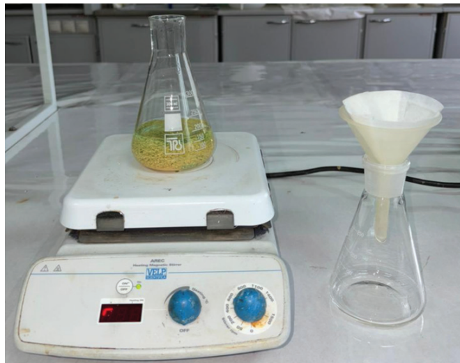
Figure 1. Scheme of the process of desilication of the sorbent and subsequent filtration.
