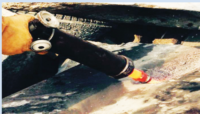
Figure 9. Operating process of the TRB-12 M1 thermal cutter with a nozzle.
