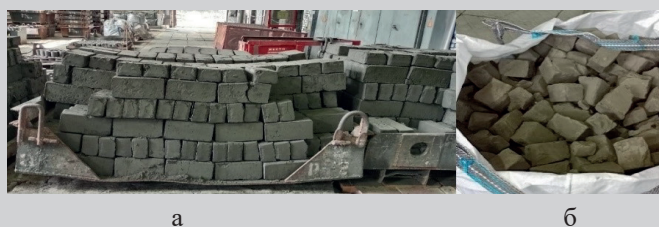
Figure 3. Appearance of dried and packaged briquettes: a) briquettes after drying; b) briquettes after packing in big bags.
